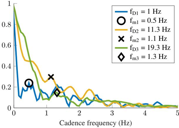
**Fig. 4:** Cadence frequencies represented by the circle, cross and diamond markers, corresponding to the Doppler bins 1 Hz, 11.3 Hz and 19.3 Hz respectively.
