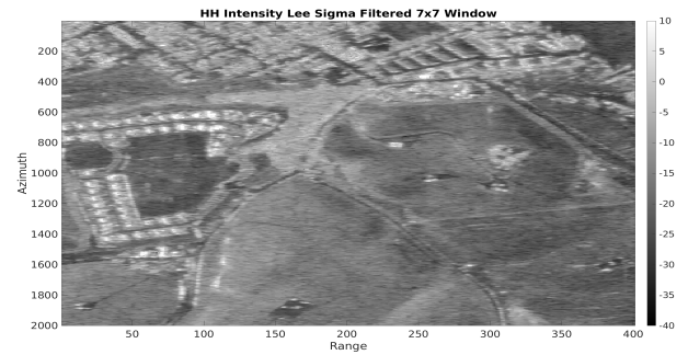
Fig. 3: HH intensity obtained using a Lee Sigma Filter with a 7x7 window in dB
