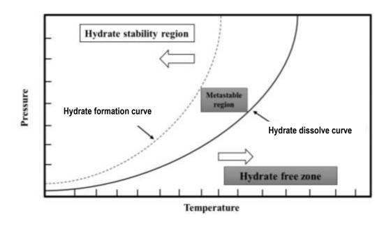
**Figure 2**: Process optimization of gas hydrate formation curve [33].
