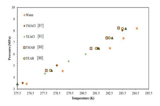
**Figure 6.** The influence of alkyl chain length of ILs at 10 wt.% concentration on phase behaviour of CH<sub>4</sub> hydrates.
