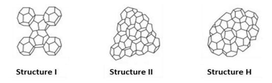
**Figure 3.** Different crystallographic structures of gas hydrates [37].
