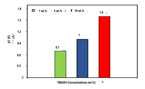
Figure 8. THI performance of [TMAOH] for mixed gas [70/30 CO<sub>2</sub>/CH<sub>4</sub> mol%] [34].
