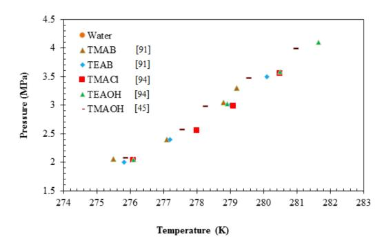
**Figure 7.** Alkyl chain length of ILs at 10 wt.% concentration on hydrate liquid vapour [HLVE] curve of CO<sub>2</sub> hydrates [44, 94, 97].
