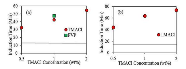
**Figure 9.** Effect of induction time on CO<sub>2</sub> hydrates at different temperature (a) 274 K (b) 277 K [88].
