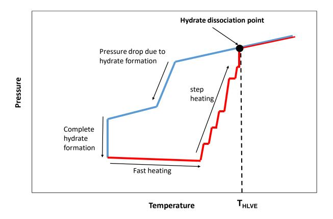
**Figure 4.** Determination of hydrate dissociation point and hydrate aqueous liquid vapor equilibrium temperature T<sub>HLVE</sub>, on a standard P-T diagram obtained through T-cycle technique (slow cooling curve in blue and step heating curve in red).
