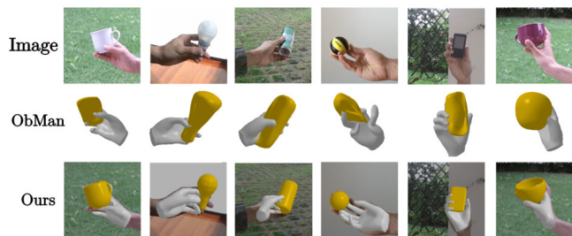
Figure 6: Comparison with [19]: Qualitative comparison of our fits to the ObMan-trained model [19] estimations on the Core50 dataset. While our model requires an approximate mesh to be provided, it generalizes to objects of arbitrary topology.
