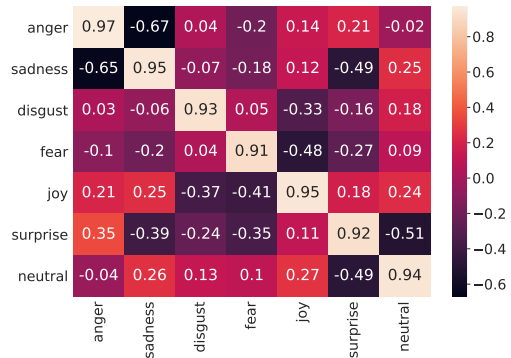
Fig. 2: Scores illustrating closeness of each expressivity class with others created using expressive similarity score computed on MSA II TTS system for speech synthesis datasets
