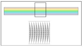
Figure 3. Flow pattern of the non-perturbated flow. Streamlines and velocity profiles in the mid-section for Re=1 and T=0.
