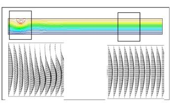
Figure 5. Streamlines and velocity profiles in two different sections for Re=1 and T=100 and M=10.
