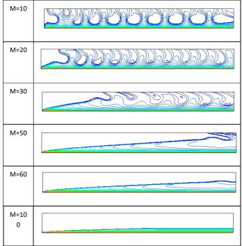
Figure 12. Snapshot of the charge density isocontours distribution at the same given time for different values of the M parameter, Re=1, T=200
