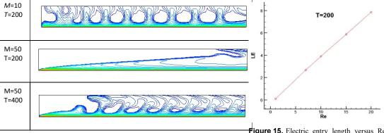
Figure 15. Electric entry length versus Reynold number for T=200 and M=10.
