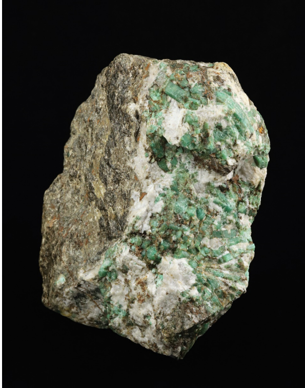
Fig. 1: Exceptional sample of emerald on matrix from Egypt, which was on exhibition at the World Exposition in 1867 (ENSMP 2115; 16 x 13.5 x 7.2 cm; crystals up to 3 cm). Crystals of emeralds are localized within a pegmatite vein within the micaschist. Photo: Musée de Minéralogie MINES Paristech / E. Gaillou.
