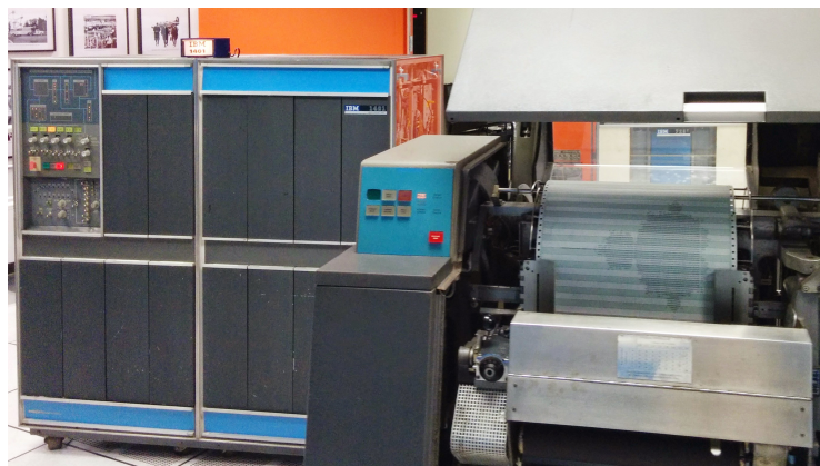
The IBM 1401 mainframe computer (left) at the Computer History Museum printing the Mandelbrot fractal on the 1403 printer (right). Photography taken from K. Shirriff's blog .
