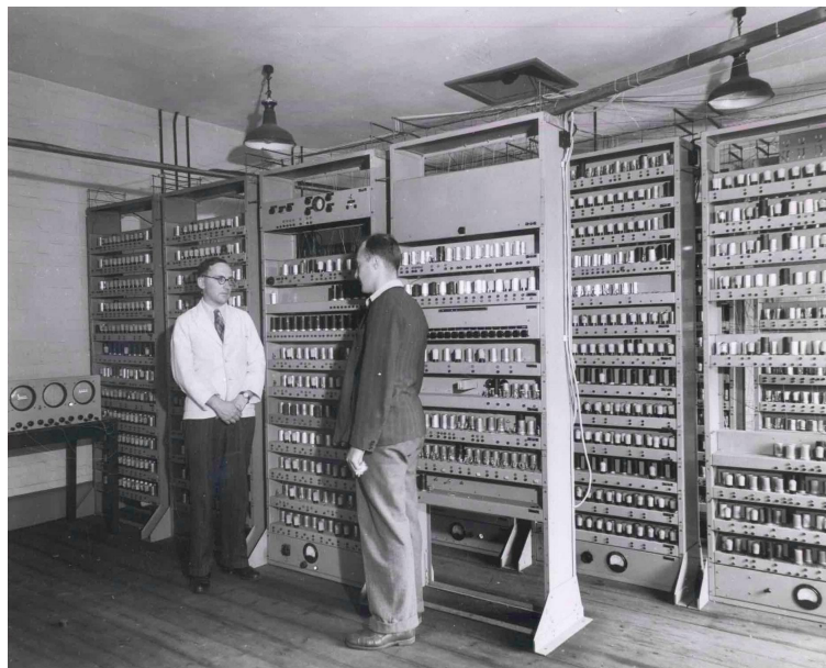
The Electronic delay storage automatic calculator (EDSAC) was an early British computer Inspired by von Neumann's seminal First Draft of a Report on the EDVAC, the machine was constructed by Maurice Wilkes and his team at the University of Cambridge Mathematical Laboratory. It was released in 1949. Source: Wikipedia .
