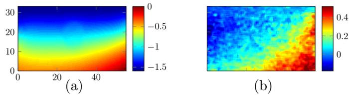
Figure 3: Example of a displacement field before regularization, obtained from a phantom experiment (CIRS model 049, Type III inclusion). (a) axial displacement,  $u_y$  (in mm), and (b) lateral displacement,  $u_x$  (in mm). In (a), axes are in millimeters.
