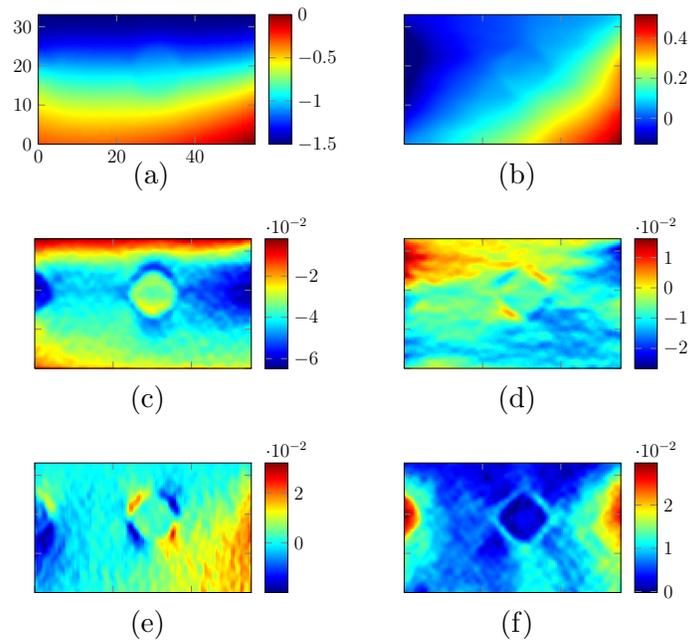
Figure 5: Displacement components after regularization and their derivatives for the CIRS model 049, Type III inclusion. (a) axial displacement,  $w_y$  (in mm), (b) lateral displacement,  $w_x$  (in mm), (c) axial strain ( $\partial_y w_y$ ), (d) lateral-shear strain ( $\partial_y w_x$ ), (e) axial-shear strain ( $\partial_x w_y$ ), and (f) lateral strain ( $\partial_x w_x$ ). In (a), axes are in mm.
