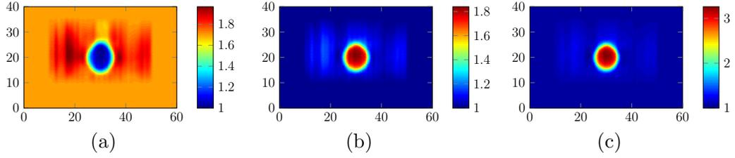
Figure 8: Relative shear modulus maps obtained with the 3D simulations, for a medium characterized by an inclusion-to-background shear modulus ratio of (a)  $4/9$  (case #4), (b)  $16/9$  (case #5), and (c)  $27/9$  (case #6). Axes are in mm.
