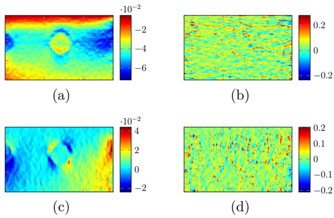
Figure 4: Derivatives of the displacement components before regularization, obtained from the fields displayed in Figure 3. (a) axial strain  $(\partial_y u_y)$ , (b) lateral-shear strain  $(\partial_y u_x)$ , (c) axial-shear strain  $(\partial_x u_y)$ , and (d) lateral strain  $(\partial_x u_x)$ .
