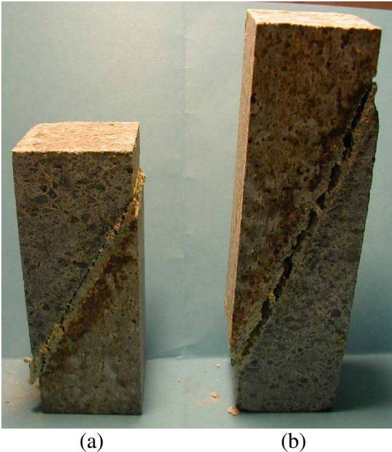
Figure 6: Failed specimens (of section 35x35 mm 2 ) with different angles of inclination after a slant shear test: (a) interface failure, (b) mortar failure.
