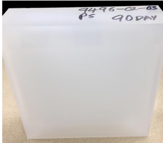
Fig. 1.9 Example of temporary fogging of PS after hot and humid exposure and rapid cooling performed in a laboratory (reproduced from [145] with permission from Elsevier)
