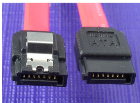
Figure 7. A poka yoke to prevent human-made operational faults induced in the system
