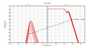
Fig. 2. Bode plots  $\left(\frac{e_f}{w_r}\right)$  and  $\frac{e_f}{w_n}$  of the frozen error systems.
