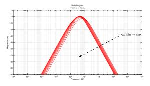
Fig. 3. Bode plots  $\left(\frac{e_f}{\Delta \Phi}\right)$  of the frozen error systems.
