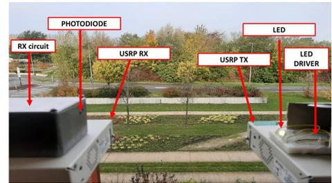
Fig. 2. Experimental Setup
