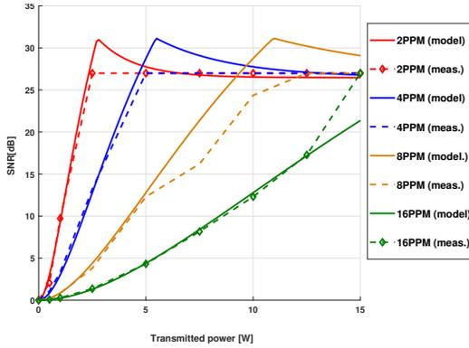
Fig. 3. Transmitted power vs Signal to Noise Ratio
