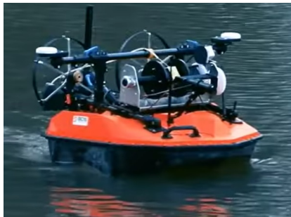
Fig. 1. The SPYBOAT® technology is based on the use of an aquatic drone allowing the realization of water sampling and inspections by guaranteeing the non-contamination of the environment.
