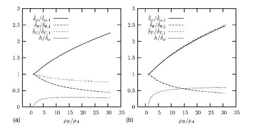
FIG. 7. Evolutions of the spreading rates and drift as functions of the density ratio. (a) Low-speed binary mixing. (b) Low-speed thermal mixing. The spreading rates are normalized by their constant-density value ( $\rho_B/\rho_A$  = 1), and the drift by the vorticity thickness.
