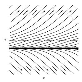
FIG. 6. Instantaneous streamlines in the coflowing mixing layer ( $\hat{u}_c$ =3). High-speed thermal mixing with A=0 and  $M_u$ =1.4. The dotted line corresponds to the z=0 axis, and the scale ratio between the x and z axis is arbitrary.
