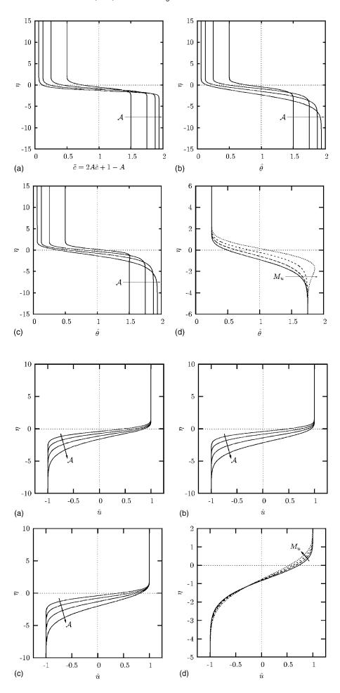
FIG. 3. Concentration or temperature profiles across the mixing layer. (a) Low-speed binary mixing, (b) low-speed thermal mixing, and (c) high-speed thermal mixing at  $M_u$ =1.4, with different values of the Atwood number. A=0.5,0.75,0.875,0.9375. (d) High-speed thermal mixing with A=0.75 and different values of the Mach number:  $M_u$ =0,1,1.5,2.
