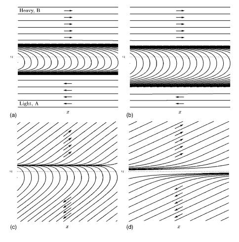
FIG. 5. Instantaneous streamlines in the mixing layer. (a) Low-speed binary mixing with A=0.75, (b) low-speed thermal mixing with A=0.75, (c) high-speed thermal mixing with A=0.75 and  $M_u$ =1.4, and (d) high-speed thermal mixing with A=0 and  $M_u$ =1.4. The dotted line corresponds to the z=0 axis, and the scale ratio between the x and z axis is arbitrary.
