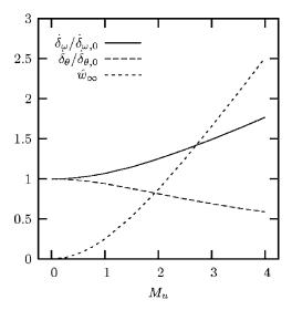
FIG. 8. Evolutions of the spreading rates and global deflection as functions of the Mach number. The spreading rates are normalized by their value at  $M_u$ =0. The deflection is quantified by the absolute value of the transverse velocity at infinity, normalized by the time-dependent velocity scale  $W_0$ .
