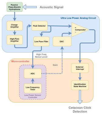
Fig. 4. Sperm Whales detector block diagram.
