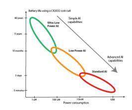
Fig. 3. Different types of embedded AI according to their power consumption
