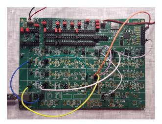
Fig. 8. Analog test and power measurement board
