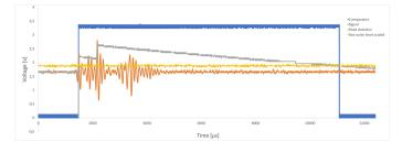
Fig. 7. Cetacean clicks signal with ultra-low power processing, acquired on real signals. Input signal high-pass filtered is in orange,  $V_{Ref}$  is in yellow, click envelope is in grey and output of the comparator is in blue.
