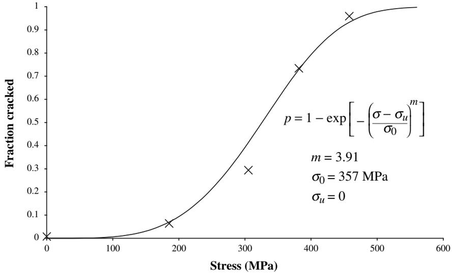
Figure 3. Fraction of cracked particles versus particle stress. Data fit to the Weibull function for determination of the Weibull modulus ( $m$ ), the characteristic stress ( $\sigma_0$ ) and the threshold stress ( $\sigma_u$ ).
