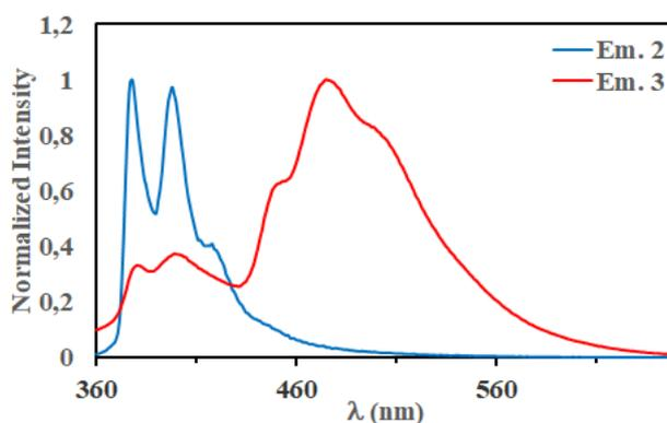
**Figure 7.** Emission bands of **2** (blue) and **3** (red) recorded in CH<sub>2</sub>Cl<sub>2</sub> at ambient temperature.
