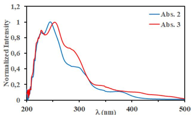
**Figure 6.** Absorption spectra of **2** (blue) and **3** (red) recorded in CH<sub>2</sub>Cl<sub>2</sub> solution at room temperature.
