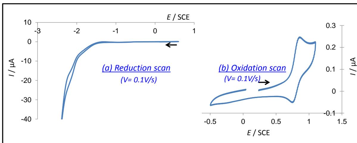
**Figure 5.** Cyclic voltammetry of complex **2** (2 mM) in  $\text{CH}_2\text{Cl}_2$  in presence of  $n\text{Bu}_4\text{NBF}_4$  (0.3M) at a platinum disk electrode (0.5 mm in diameter) and at a scan rate of  $0.1 \text{ V}\cdot\text{s}^{-1}$ . (a) Cathodic scan and (b) anodic scan.
