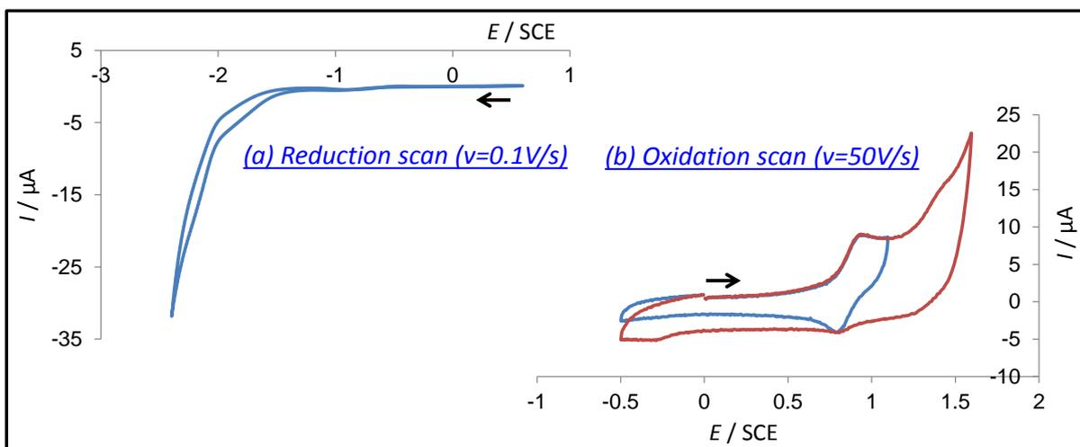
**Figure 4.** Cyclic voltammetry of complex **3** (2 mM) in  $\text{CH}_2\text{Cl}_2$  in presence of  $n\text{Bu}_4\text{NBF}_4$  (0.3M) at a platinum disk electrode (0.5 mm in diameter). (a) Cathodic scan at  $0.1 \text{ V}\cdot\text{s}^{-1}$  and (b) anodic scan at  $50 \text{ V}\cdot\text{s}^{-1}$ .
