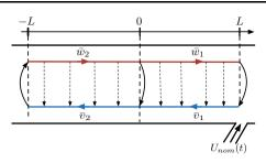
FIGURE 3 Traffic flow on an incoming road and an outgoing road connected with a junction. Actuation is implemented at the outlet with ramp metering.
