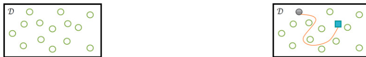
Fig. 1: Sampling for optimization in parameter space D . (a) Apriori sampling D_s . (b) Adaptive sampling, ● initial parameters, ■ optimal parameters, — optimization trajectory, ○ sample parameters.
