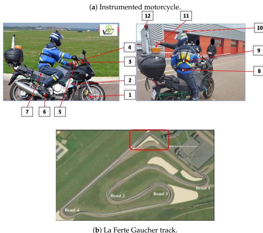
Figure 1. The heavily instrumented motorcycle and the La Ferte Gaucher track
