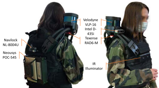
Fig. 2. Tactical waistcoat hardware configuration.
