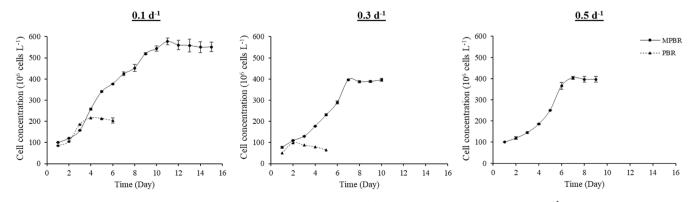
**Fig. 2.** Growth kinetics of *Haslea ostrearia* in PBR ( $\blacklozenge$ ) and MPBR ( $\blacklozenge$ ) operating at different dilution rates of 0.1, 0.3 and 0.5 d<sup>-1</sup>. Washout occurred in the PBR, indicated by the continuous decrease of the cell concentration. Results were expressed as mean  $\pm$  standard deviations of triplicate determinations.
