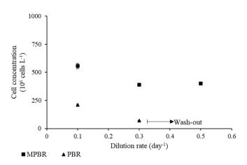
**Fig. 3.** Stabilized cell density of *Haslea ostrearia* in both PBRs operating at different dilution rates. Washout in PBR ( $\blacklozenge$ ) at dilution rate D equal to 0.3 d<sup>-1</sup>. MPBR ( $\blacksquare$ ) was able to prevent washout up to D = 0.5 d<sup>-1</sup> allowing higher cell concentration. Results were expressed as mean  $\pm$  standard deviations of triplicate determinations.
