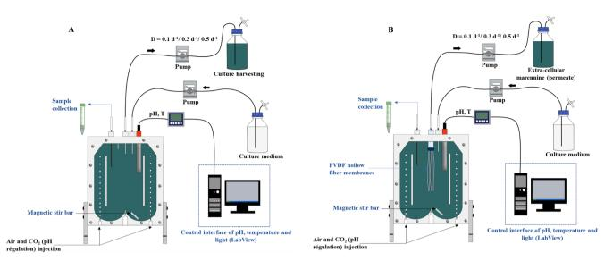
**Fig. 1.** The schematic illustration of the microalga cultivation process using MPBR and PBR. A) PBR without membrane filtration, B) PBR with membrane filtration. Both of them are operated at different dilution rate (D) equal to 0.1, 0.3 and 0.5 d<sup>-1</sup>. Before sampling stirring with a magnetic bar on the photobioreactor walls as well as manual stirring of fiber bundle was carried out.
