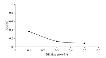
Fig. 6. Membrane retention rate with the MPBR operating at different dilution rates.
