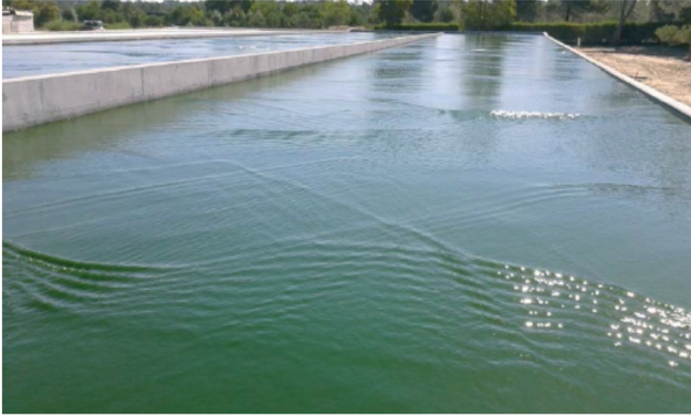
Fig. 7 Cascade of inclined plane photobioreactor of A4F in Pataias, Portugal (reproduced with the permission of A4F company, www.a4f.pt).
