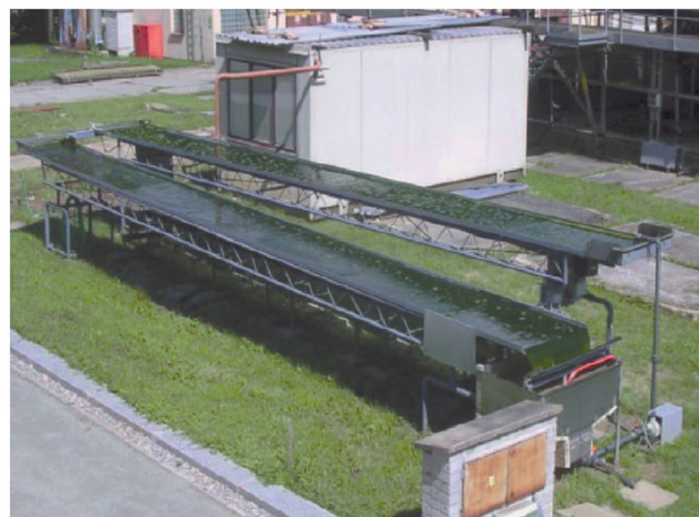
Fig. 6 Inclined plane system (200 litres) developed in Trebon, Czech Republic 68 (original figure was published in J. R. F. Malapascua, C. G. Jerez, M. Sergejevová, F. L. Figueroa and J. Masojidek, Aquat Biol. , 2014, 22, 123–140, under the Creative Commons CC-BY License).
