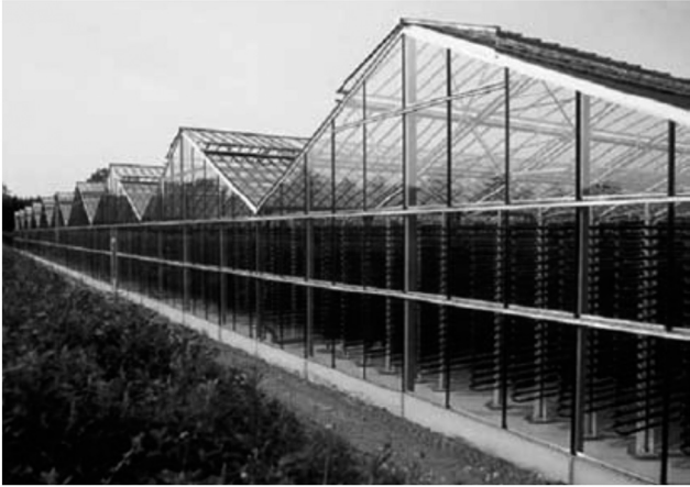
Fig. 8 Tubular photobioreactor in greenhouse in Klötze, Germany 69 (agreement from Springer Nature in the framework of Copyright Clearance Center).
