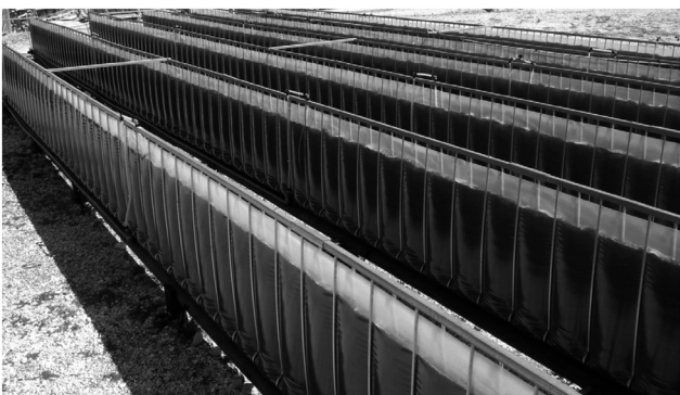
Fig. 9 PBR green wall panels in Siesto Fiorentino, Italie 80 (this figure was published in M. R. Tredici, N. Bassi, M. Prussi, N. Biondi, L. Rodolfi, G. Chini Zittelli and G. Sampietro, Applied Energy , 2015, 154(September), 1103–1111, Copyright Elsevier).
