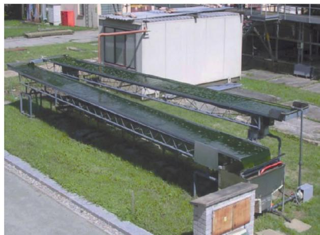
Fig. 6 Inclined plane system (200 litres) developed in Trebon, Czech Republic<sup>68</sup> (original figure was published in J. R. F. Malapascua, C. G. Jerez, M. Sergejevová, F. L. Figueroa and J. Masojidek, *Aquat Biol.*, 2014, 22, 123–140, under the Creative Commons CC-BY License).
