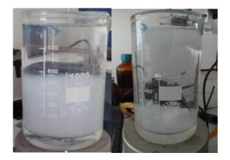
Fig. 5.Visual aspect of the water after treatment (5a left side) without pH adjustment (5b right side) and with continuous pH adjustment every 30 minutes ( $i = 10 \text{ mA} \cdot \text{cm}^{-2}$ ,  $[PO_4^{3^-}]_i = 100 \text{ mg} P.L^{-1}$ , [NaCl] = 6.5 mM,  $pH_i = 7$ , T = 30 °C)
