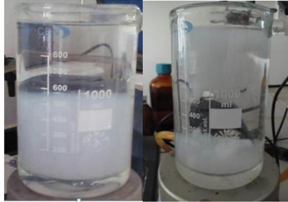
Fig. 5. Visual aspect of the water after treatment (5a left side) without pH adjustment (5b right side) and with continuous pH adjustment every 30 minutes (  $i = 10 \text{ mA} \cdot \text{cm}^{-2}$ ,  $[\text{PO}_4^{3-}]_i = 100 \text{ mg P} \cdot \text{L}^{-1}$ ,  $[\text{NaCl}] = 6.5 \text{ mM}$ ,  $\text{pH}_i = 7$ ,  $T = 30 \text{ }^\circ\text{C}$  )
