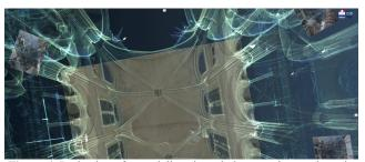
Figure 4: Projection of a spatially oriented photograph onto the point cloud of the Notre-Dame de Paris cathedral displayed within the 3D viewer developed by the MAP laboratory as part of the scientific action for the reconstruction of the Notre-Dame de Paris cathedral. (Violette Abergel, Livio De Luca)
