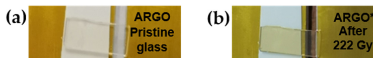
Figure 2. (a) Transparent color before irradiation (ARGO glass sample), (b) yellow color after X-ray irradiation with 222 Gy (ARGO* glass sample).
