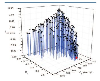
**Figure 5.** Approximate Pareto front of extractive distillation design for acetone—methanol—water system,  $E_{\text{ext}}$  versus  $R_1$  and  $F_E$ . The red diamond indicates G1.
