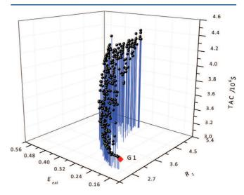
**Figure 4.** Approximate Pareto front of extractive distillation design for acetone—methanol—water system, TAC versus  $E_{\text{ext}}$  and  $R_1$ . The red diamond indicates G1.
