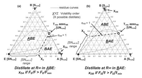
Figure 3. Thermodynamic features of 1.0-1a mixtures. Separation of a minimum boiling azeotrope with a heavy entrainer (adapted from Shen et al. <sup>14</sup>).
