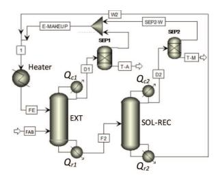
Figure 1. Extractive distillation flow sheet.
