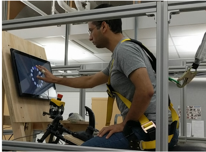
(a) A subject completing Task 1 selections using a braced posture in the force condition. The joystick used for Tasks 2 and 3 is also visible.
