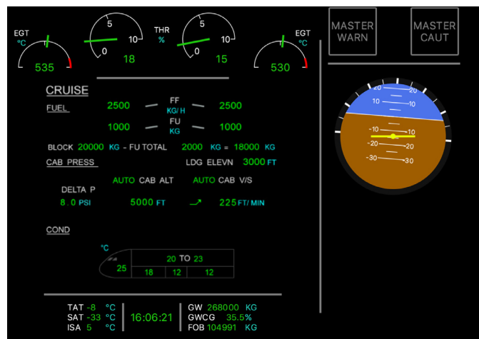
Fig. 7. Task 2 interface, including touchscreen-adapted Centralised Aircraft Monitoring and Crew Alerting (CAMCA) and Attitude Indicator (AI, right).
