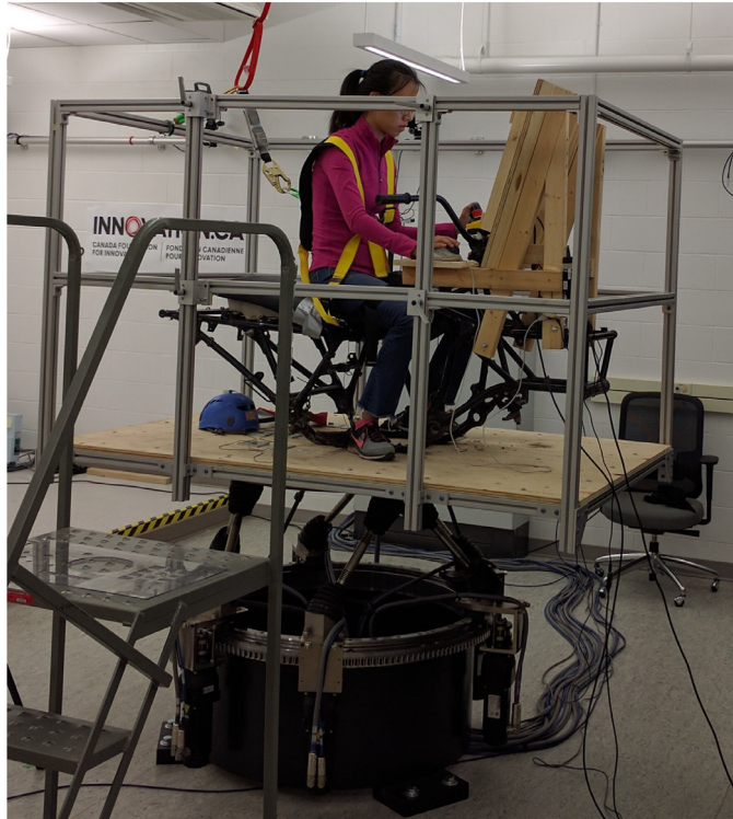
(b) A Mikrolar R-3000 rotopod motion platform induced vibration.
