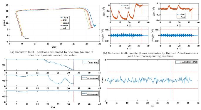
(c) Software fault: the agreement indicators of the Euclidean distance of (d) Software fault: The residues of the Euclidean distance measured by the first and second Kalman filters and the DM the first GPS and the second GPS
