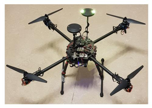
Figure 15: Experimental Tarot 650 quadrotor
