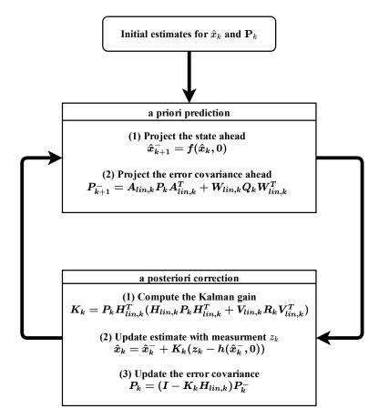
Figure 7: Data flow of the Extended Kalman filter operation
