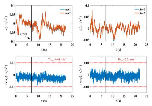
Figure 20: GPS additive fault: accelerations estimates by the two Accelerometers and their corresponding residues
