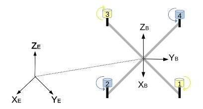
Figure 2: Quadrotor configuration
