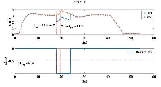
Figure 22: Lidar additive fault: The measured altitude and the residues of the Lidar's output used in KF1 and KF2
