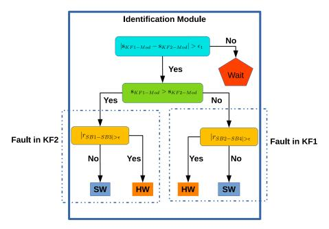
Figure 14: Proposed data fusion architecture for tolerating sensors and software faults
