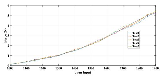
Figure 4: Thrust force as function of the applied PWM input
