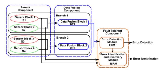
Figure 1: Duplication-comparison architecture for fault tolerance in multi-sensor data fusion, adopted from [1]
