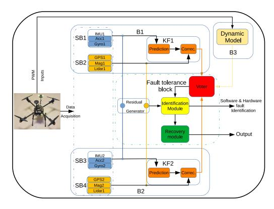
Figure 8: Proposed data fusion architecture for tolerating sensors and software faults
