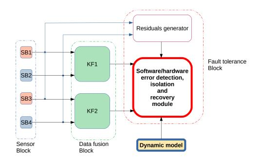
Figure 11: Fault tolerance architecture using Duplication comparison and analytical redundancy
