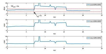
Figure 19: GPS additive fault: The residues of the x, y, d components between the first GPS and the second GPS
