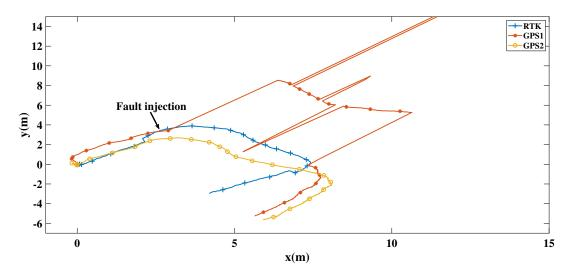
Figure 18: GPS additive fault: positions measurements of the two GPS and the RTK GPS  $% \left( {{\rm GPS}} \right)$
