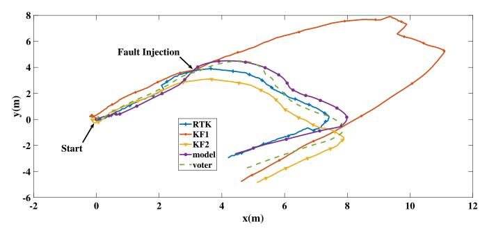
Figure 16: GPS additive fault: positions estimated by the two Kalman fi lters, the dynamic model, the voter, and the ground truth given by a GPS RTK
