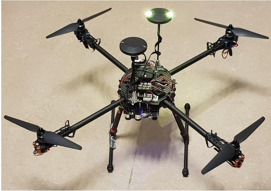
Figure 15: Experimental Tarot 650 quadrotor
