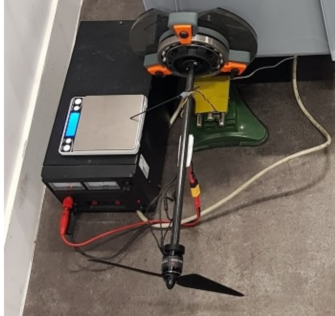
Figure 5: Experimental setup for torque identification of the Tarot 650
