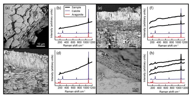
**Figure 3.** SEM images and Raman spectra for a selection of samples. (**a**, **c**, **e**, and **g**) SEM images of samples POL-8, POL-12, ARD-05, and ARD-03, respectively. (**b**, **d**, **f**, and **g**) Raman spectra of samples POL-8, POL-12, ARD-05, and ARD-03 compared to the reference spectra of calcite and aragonite.
