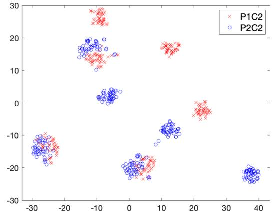
Fig. 7. Impact of press signature. Comparison of samples printed using the same engraved cylinder ( $C_2$ ) but using two presses ( $P_1$  and  $P_2$ ). For each cylinder there is six clusters, one for each regular pattern position. Clusters highlighted in red (resp. blue) belongs to the class  $P_1C_2$  (resp.  $P_2C_2$ ).
