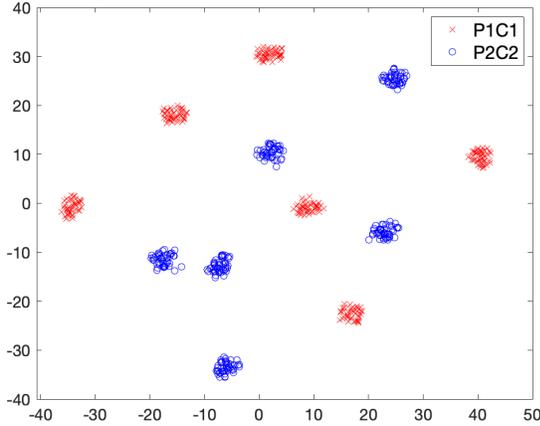
Fig. 9. Impact of cylinder and press signatures. Comparison of samples printed using two engraved cylinders ( $C_1$  and  $C_2$ ) and two presses ( $P_1$  and  $P_2$ ). For each cylinder there is six clusters, one for each regular pattern position. Clusters highlighted in red (resp. blue) belongs to the class  $P_1C_1$  (resp.  $P_2C_2$ ).
