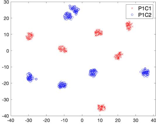
Fig. 8. Impact of cylinder signature. Comparison of samples printed using two engraved cylinders ( $C_1$  and  $C_2$ ) and one press ( $P_1$ ). For each cylinder there is six clusters, one for each regular pattern position. Clusters highlighted in red (resp. blue) belongs to the class  $P_1C_1$  (resp.  $P_1C_2$ ).
