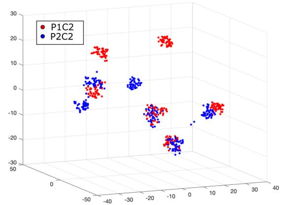
Fig. 11. Impact of press signature in 3D visualization. Comparison of samples printed using the same engraved cylinder ( $C_2$ ) but using two presses ( $P_1$  and  $P_2$ ). For each cylinder there is six clusters, one for each regular pattern position. Clusters highlighted in red (resp. blue) belongs to the class  $P_1C_2$  (resp.  $P_2C_2$ ).
