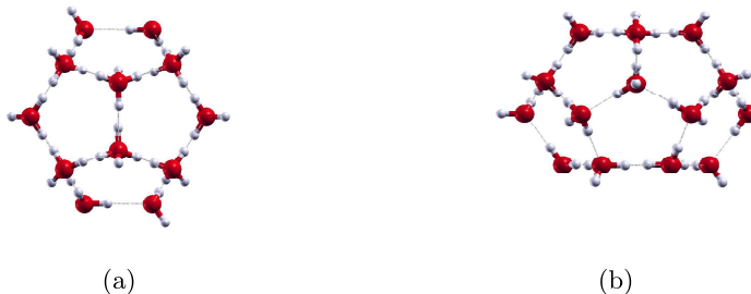
Figure 1: Optimized geometries of empty (a) small ( 5^{12} ) and (b) large ( 5^{12}6^2 ) cages of sI clathrate.
