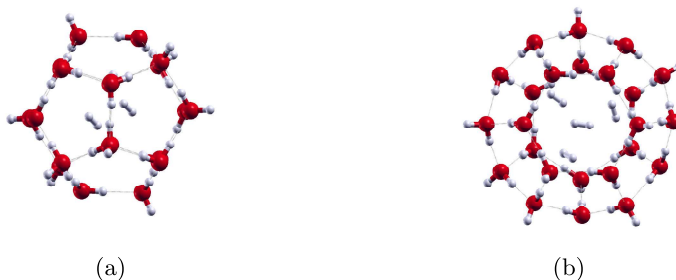
Figure 2: Optimized configurations of H_2 molecules at optimum cage occupancies inside (a) small ( 5^{12} ) and (b) large cages ( 5^{12}6^2 ) of sI clathrate.
