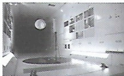
ColKa antenna being tested in the Hertz Test Chamber of ESA/ESTEC. The blue spikes isolate the room from electromagnetic interference, recreating the radio frequencies of space. Image credit: ESA, M. Cowan.
