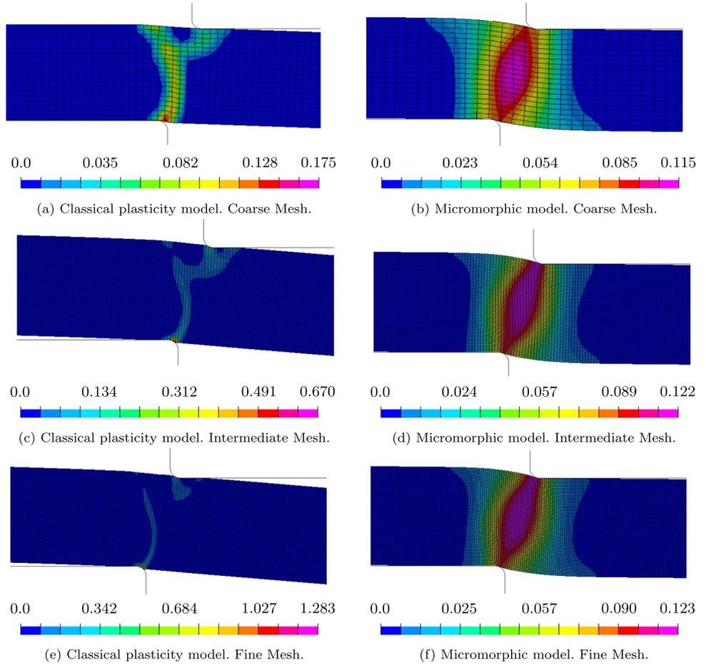
and **e** by the contours of the cumulative plastic strain. The magnitude of the cumulative plastic strain is different for two different mesh discretizations, and it increases with
