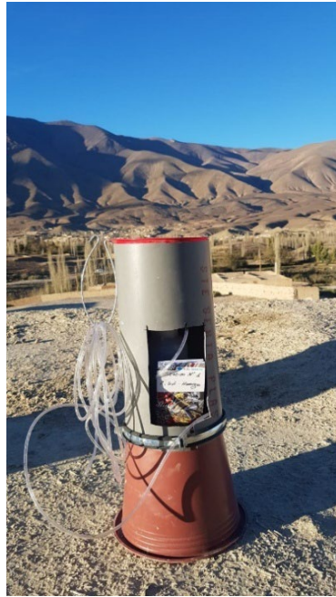
Figure 3. Rain collection system.
