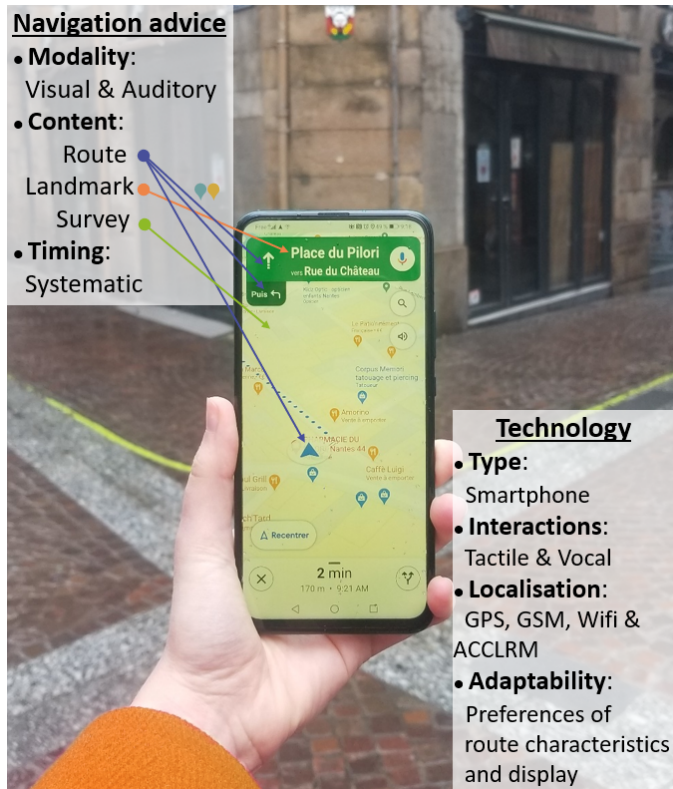
Fig. 1. Example of a commercially available navigation device and its characteristics in terms of technology and navigation advice.
