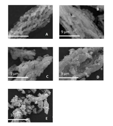
Fig. 3. SEM images of the  $TiO_2 - SiO_2$  composites obtained from SBA-15 aged at 130 °C (series b) with 10 wt% (A), 25 wt% (B), 50 wt% (C), 70 wt% (D) and 80 wt% (E) of  $TiO_2$ .
