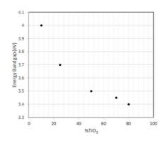
Fig. 13. Evolution of the energy band gap of the composites according to the  $TiO_2$  content.
