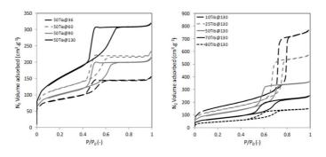
Fig. 5. N<sub>2</sub> adsorption – desorption isotherms of the composites.
