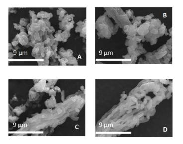
Fig. 2. SEM images of the 50 wt% TiO<sub>2</sub> - SiO<sub>2</sub> composites (series a) obtained from SBA-15 aged at different temperatures.
