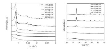
Fig. 9. Low angles (left) and wide angles (right) XRD patterns of the catalysts with different TiO<sub>2</sub> content (series b).
