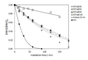
Fig. 14. Evolution of MO concentration with irradiation time by using the different catalysts at 50 wt% of TiO<sub>2</sub> (series a) and two commercial references.
