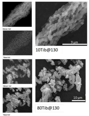
Fig. 4. SEM and corresponding elemental mapping images of 10Tib@130 and 80Tib@130.
