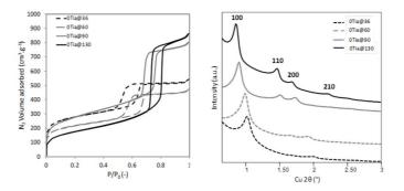
Fig. 1. N<sub>2</sub> adsorption – desorption isotherms (left) and low-angles X-ray diffraction patterns (right) of SBA-15 type mesoporous silicas synthesized after ageing at different temperatures.
