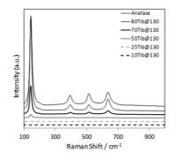
Fig.10. Raman spectra of the composites of series b
