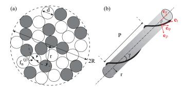
FIG. 3. (a) Section of a yarn of radius R composed of fibers of diameter d. Gray fibers go downwards and white fibers go upwards. (b) A fiber twisted on a cylinder of radius r.
