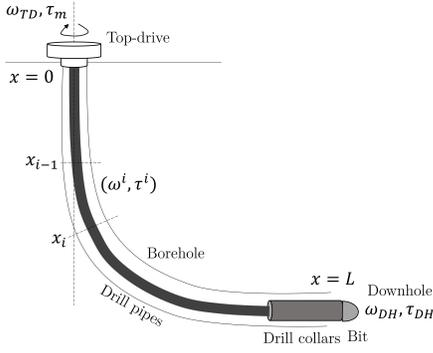
Fig. 1. Schematic drill string in a deviated borehole.
