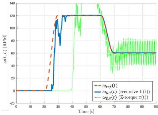
Fig. 3. Evolution of the downhole angular velocity.
