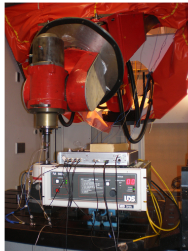
Figure 13. First natural frequency measurement.
