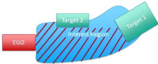
Fig. 1. Example of implementation of the metric, we build the zone of danger here in blue according to the dynamic parameters of the vehicle and we look at the space that remains once we remove the space made inaccessible by the targets around the ego.
