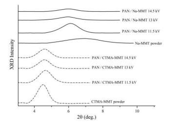
Figure 7 XRD patterns of pristine Na-MMTC16TMA-MMT, PAN/Na-MMT obtained at different voltages and C16TMA treated PAN/Na-MMT samples
