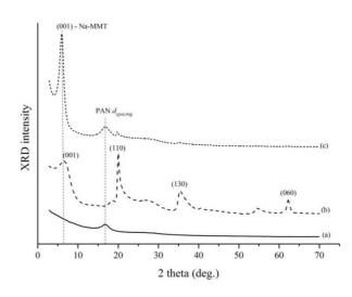
Figure 6 XRD patterns of PAN nanofibers (a), Na-MMT powder (b) and nanofibers of PAN filled with 19 wt% Na-MMT. (Nanofibers are produced at 11.5 kV)
