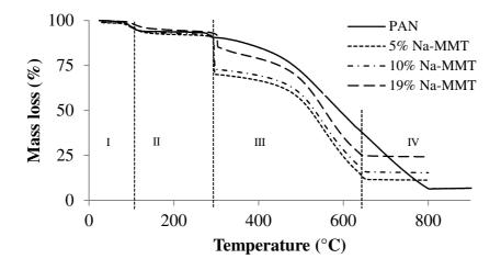
Figure 3 TGA curves of PAN and PAN/Na-MMT nanofibers
