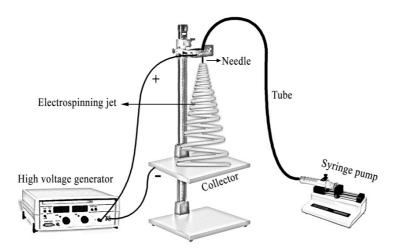
Figure 1 Scheme of the home-made Electrospinning setup
