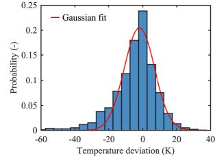
**Figure 8** - Histogram of difference between the 70,000 single-shot temperature and the temperature found with the LMS method. Bar width is 5 K. A Gaussian fit is applied with 95% confidence bounds resulting in an average temperature deviation of  $\mu = -1.97$  K and a standard deviation of  $\sigma = 12.59$  K.
