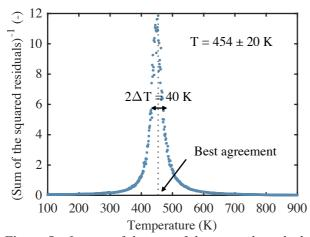
**Figure 5 -** Inverse of the sum of the squared residuals between a single-shot spectrum and average spectra from the database as a function of temperature.
