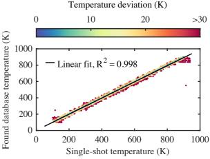
**Figure 7 -** *Scatter plot of the temperature found with the LMS method and the recorded single-shot temperature. The color indicates the absolute temperature deviation.*
