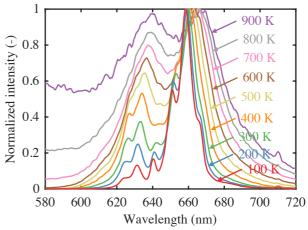
**Figure 2 -** Normalized average Mg<sub>3.5</sub>FGeO<sub>5</sub>:Mn phosphorescence spectra at different temperatures after laser excitation at 355 nm with a fluence of 106 mJ.cm<sup>-2</sup>.
