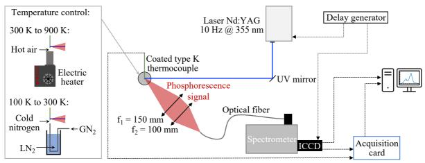
Figure 3 - Experimental setup for phosphorescence spectra acquisition from 100 K to 900 K.
