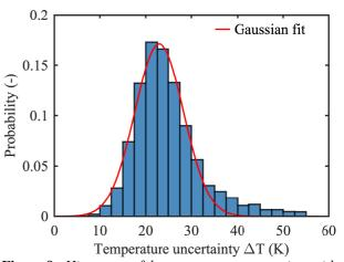
**Figure 9** - Histogram of the temperature uncertainty with the LMS method applied on the 70,000 single-shots spectra. Bar width is 5 K. A Gaussian fit is applied with 95% confidence bounds resulting in an average temperature uncertainty of  $\mu = 22.95$  K and a standard deviation of  $\sigma = 15.11$  K.
