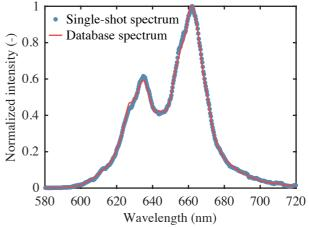
**Figure 6** – Normalized single-shot spectrum and average spectrum at 454 K extracted from the database using the LMS method.
