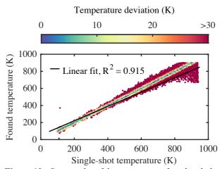
**Figure 10 -** *Scatter plot of the temperature found with the intensity ratio method and the single-shot temperature. The color indicates the absolute temperature deviation.*
